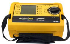
The METRISO® 3000 is a digital high resistance tester capable of measuring point-to-point resistance and resistance-to-ground measurements with a large test range of 1 kOhm to 1,2 TOhm. The meter includes an integrated data logger with a USB communication port for data transmission, temperature and relative humidity sensor, PC software for Windows, two disk probes, a hand-held probe with connecting cable, and a conductive carrying case fitted with dissipative pink foam.
