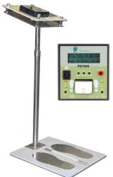
Comprehensive, accurate tool to fully meet your daily ESD checking needs. Independently tests the left and right foot along with wrist band. Innovative LCD screen will instantly display the test result and the measured resistances. The proactive "Near-Fail" indicator alerts the user that the ESD grounding device under test
