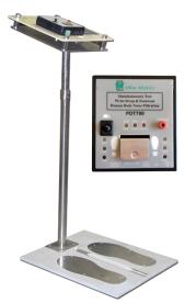
Easy, accurate, and time saving one-touch digital ground tester. Simultaneously and independently test both feet and a wrist strap while filtering out human body noise. The proactive "Near-Fail" indicator alerts the user that the ESD grounding device under test is nearing failure levels.
