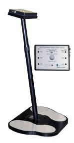
Deluxe three-state touch tester designed for fast and accurate testing of ESD ground devices. A unique dual test circuit eliminates the need for separate wrist-strap and foot grounder testers which saves money and space. Both feet can be tested at the same time.
