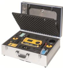
The ESD Audit Kit includes the relevant test instruments and equipment needed to perform ESD audits according to ANSI ESD20.20 and IEC 61340-5-1 and for qualification and verification of ESD control elements. Choose between the MetrisoB530 standard resistance meter or the
